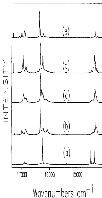
Fig 1. Room Temperature emission spectra from (a) \text{EuCl}_3 , (b) \text{EuCl}_3 \cdot \text{H}_2\text{O} , (c) \text{EuCl}_3 \cdot 2\text{H}_2\text{O} , (d) \text{EuCl}_3 \cdot 3\text{H}_2\text{O} , and (e) \text{EuCl}_3 \cdot 6\text{H}_2\text{O} .
